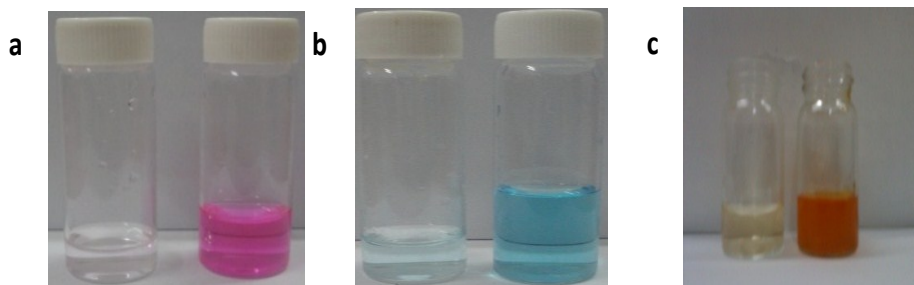
Figure 8. Photograph of dye solution(a) Rhodamine B,(b) methylene blue,(c)methyl orange before (right) and after (left) stirring.
